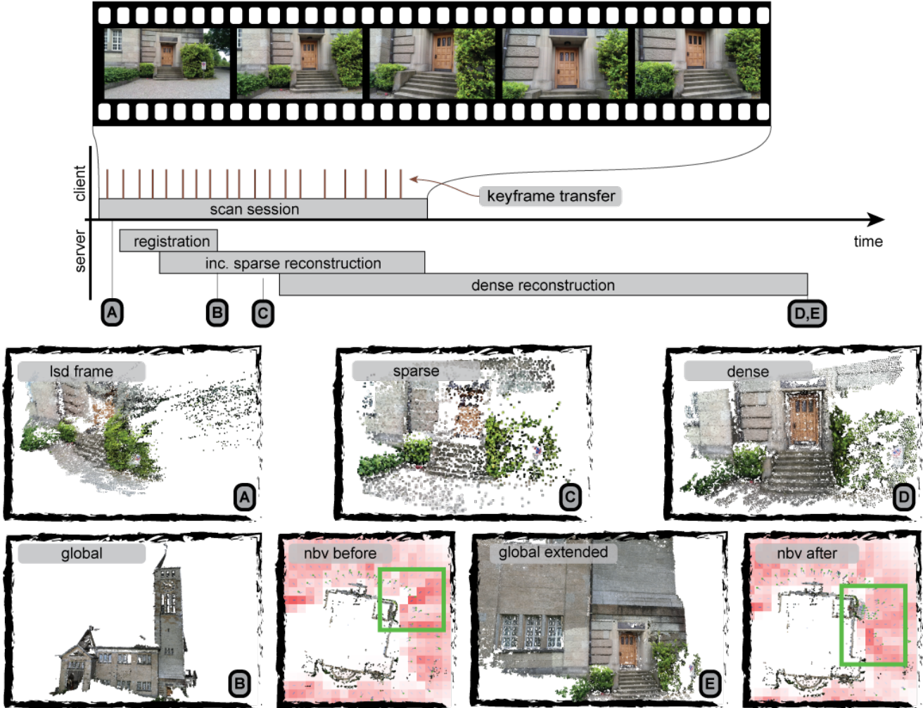
Figure 4: A timeline of a sample sequence processed by our system. During the scan session on the mobile phone, keyframes (indicated by peaks) are transferred to the remote server, where an immediate registration to a global model is started. In parallel a sparse reconstruction only of the session model delivers an accurate sparse point cloud, which again is densified on the cloud. The middle row shows the visual feedback, available to the client at different time steps. If global registration succeeds, a dense version of the whole surrounding is presented immediately and afterwards extended by the new images (bottom row). A next best view (nbv) map, indicates good spots for additional images with red peaks.
