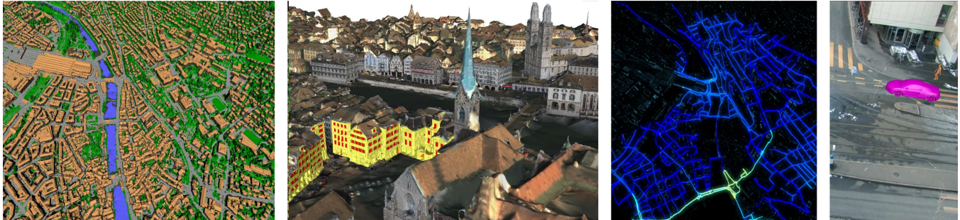
Figure 1: Data used in our video. First: distant view of automatic city-scale 3D reconstruction with semantic segmentation of its composition into buildings, roads, vegetation, and water. Second: closer view of the textured 3D model with overlaid building-level semantic segmentation into facades, windows, balconies, and roofs. Third: distant view of a traffic model estimated for a specific hour in a weekday, based on public webcam footage. Fourth: closer view of the city’s liveliness model where avatars simulate the actual data, preserving people’s privacy.
