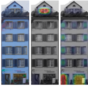
Figure 3: Heatmap representation of measured unusualness. Left: facade image, Middle: using LOF results, Right: after mapping according to human perception.
