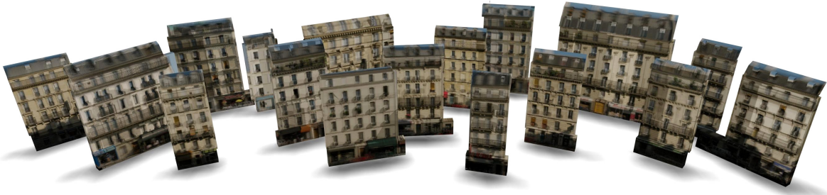
Figure 7. Estimated 3D facades. All reconstructed facades in the RueMonge2014 test set. Our method performs automatic separation of facades and analyzes the 3D structure of facade elements. The final results are obtained by fitting 3D boxes to the discovered objects and texturing with ortho-images. Please zoom in to view 3D structure, or consult the detailed view in Figure 8.
