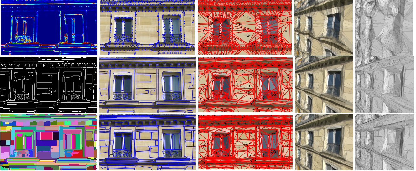
Figure 3. Different ways to obtain 2D image-aligned triangle mesh. Rows: (a) Delaunay Triangulation (DT) over image corners, (b) constrained DT over polygonized gradient edges, (c) constrained DT over polygonized superpixel boundaries. Columns: (1) Harris cornerness score / Canny edge map / superpixel label map, (2) original image with Harris corners and polygonized boundaries in blue, (3) constrained Delaunay triangulation over its mean-color rasterization (visible SfM points as black crosses), (4-5) 3D reconstruction obtained from sparse SfM data with our method introduced in Section 3.2.
