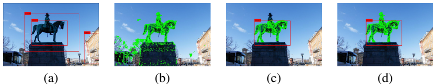
Figure 3: Object segmentation takes the object detections (a) and 3D model, visualised here by the projected points, (b), and jointly estimates the object segmentation and best detection in each image (c). We refine the segmentation, re-attaching the head in this case (d).
