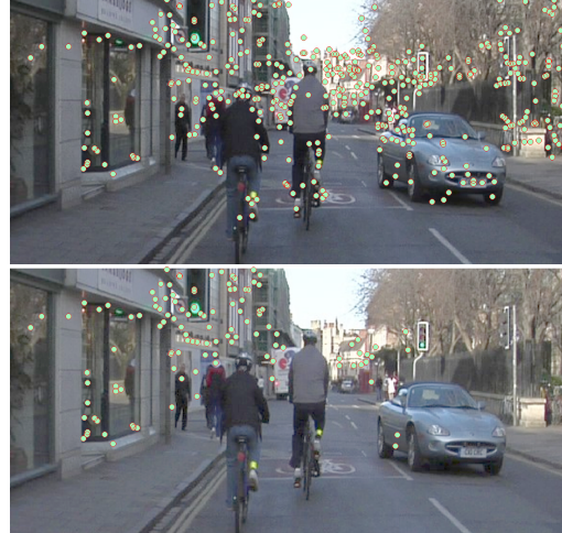
Figure 2: Search space reduction by correct matchability: The top image shows initial image features, while in the bottom only the features predicted to be matched correctly are shown. The majority of features on unreliable objects (pedestrians, car, vegetation) are omitted from the prediction, while features on buildings are preserved.
